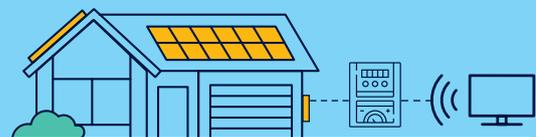
Remotely turn off the customer inverter via an AMI meter
